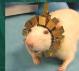
Miniature Mobile PET camera and MRI Scanning Techniques for Brain Imaging in Mice/Rats without Anesthesia
